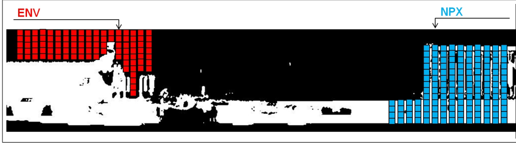
Figure 6: Illustration of the calculation of the ENV and NPX signals. Red bars correspond to the ENV signal and indicate the sum of pixels 'on top' of the last foreground pixel. Blue bars represent the NPX signal indicating the sum of foreground pixels per image column.
