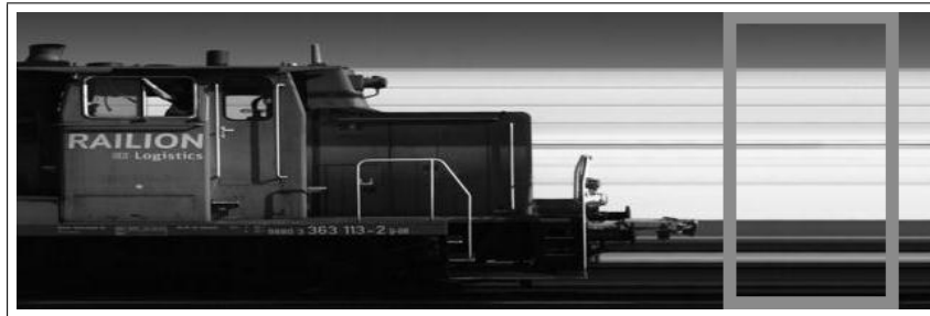
Figure 8: Start / End detection: Grey rectangle illustrates an example patch sampled from the input stream
